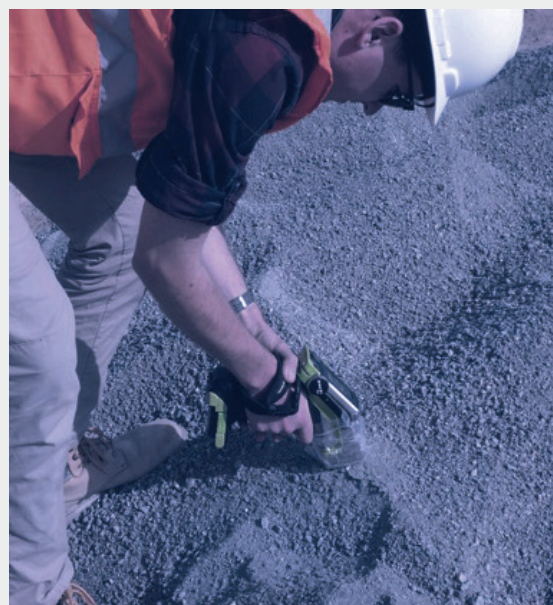
An operator scanning crushed material with the xTrace™ device at Yacari processing plant.
