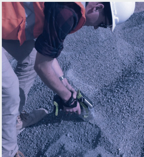
An operator scanning an ore stockpile with the xTrace™ device at Yacari processing plant.
