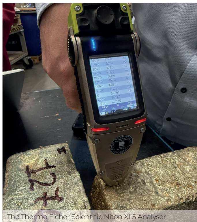
At Argor-Heraeus' premises, aXedras' team performs non-destructive analysis on Soleil Metals' doré bars using the Niton XL5 Analyser
